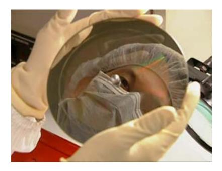
Since the glass master is too fragile to be used as an injection mold, a metal mold called a stamper is usually used.
