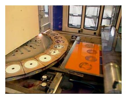
With all the steps so far a working CD has been made. The CD can then be silkscreen or offset printed with artwork. Silkscreen is normally used for vector graphics for better color matching. Offset is used for photographic artwork using CMYK as the basic color elements. Once the artwork is printed, the disk will be exposed to a high intensity UV lamp which dries the ink instantly. The discs are stacked and then transported for packaging.
